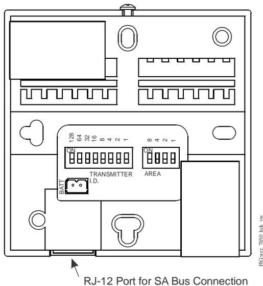
**Figure 1: TRANSMITTER ID and AREA DP Switch Blocks on a WRZ-7860-0 Receiver**
