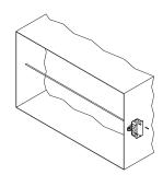
**Fig. 7**: 50/50 Vertical Stratification - Rigid Averaging Sensor Horizontal Installation
