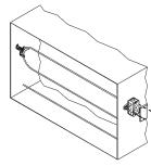
Fig. 6: Vertical Stratification -Three Pass Horizontal Installation
