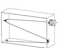
**Fig. 5**: Vertical Stratification -Three Pass Angled Installation
