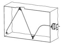
Fig. 3: Horizontal Stratification -Three Pass Angled Installation
