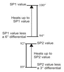
In this example, both stages are set to HEAT, but the stages are separated by 2 degrees.
