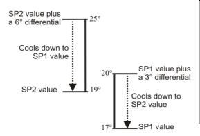
With both stages in the cooling mode, one can "stage" cooling phases. The example on the left shows stage 1 turning on to cool to bring the temperature down to 17°. If the temperature continues to rise for some reason, stage 2 kicks in at 25° to boost the cooling down.
