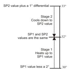
It is possible to maintain a very tight temperature range by setting one stage as a cooling stage and one stage as a heating stage.
