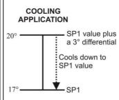
In this Cooling Application Example, the user wants to maintain a 17° temperature. With a 3° differential, SP1 value plus a 3° differential temperature to rise to 20° and then turn on the cooling application until the temperature reaches 17°. Once the temperature reaches the set point, the relay will open again and allow it to rise to 20° before starting the cycle again.
