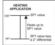
In this Heating Application Example, the user wants to maintain a 100° temperature. With a 2° differential, the controller will allow the temperature to drop to 98° and then turn on the heating application until the temperature reaches 100°. Once the temperature reaches the set point, the relay will open again and allow it to cool down to 98° before starting the cycle again.
