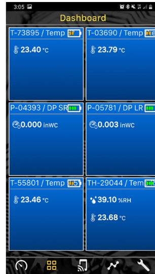
**Dashboard** - Location where up to 6 probes can be displayed simultaneously with their current readings.
