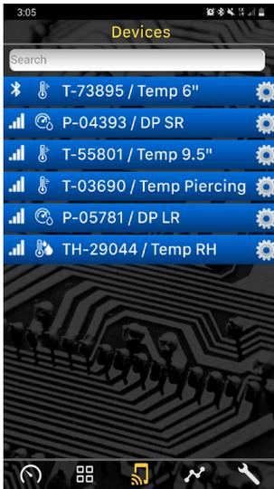
**Devices** - Lists all probes that are in communication with the app. Select probes to view live data or logs to graph or share.
