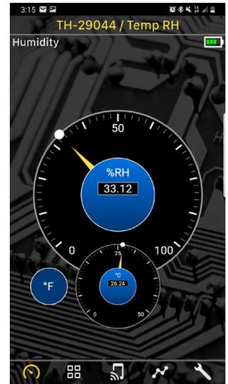
**Gauge** - Screen where one device can be displayed on a traditional gauge for easy viewing.
