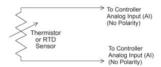
Fig. 9: 2-Wire Termination for Thermistor or RTDs
