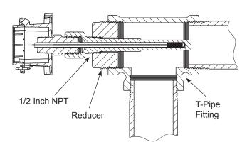
Fig 7: Typical Corner Mount (shown with Junction Box enclosure
