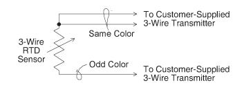
Fig. 10: 3-Wire Termination for RTDs
