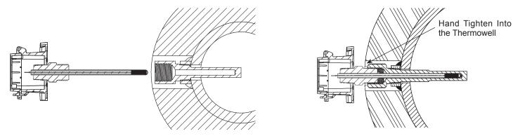
Fig 5: BAPI-Box Crossover Unit Before Insertion
