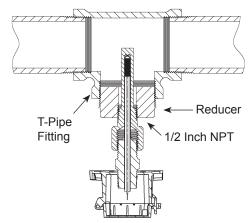
Fig 8: Typical T-Mount (shown with Junction Box enclosure
