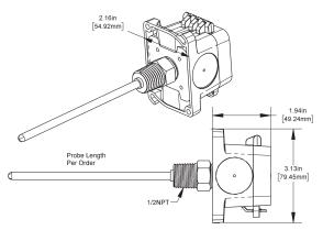
Fig 1: BAPI-Box Crossover Immersion with Stainless Steel Fittings above. Outside Mount version shown at right.
