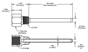
Fig 3: Two-Part Welded Thermowell
