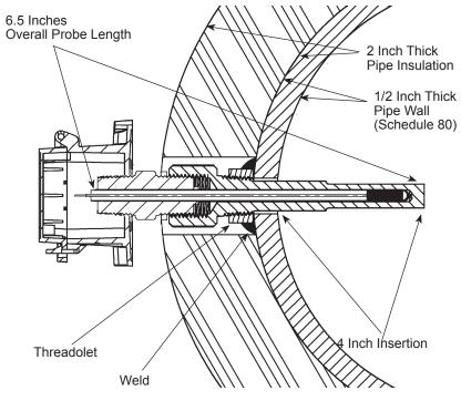
Fig 4: Typical Sensor and Thermowell Installation
