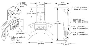
Fig. 7: Flexible Probe Bracket (BA/FPB)
