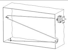
**Fig. 2:** Flexible Sensor Horizontal Mount (Best for Vertical Stratification)
