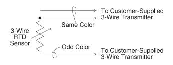
Fig. 9: 3-Wire Termination for RTDs
