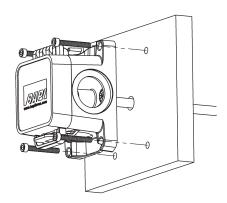
Fig. 4: BAPI-Box Crossover Mounting to the Duct
