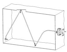
**Fig. 3:** Flexible Sensor Vertical Mount (Best for Horizontal Stratification)
