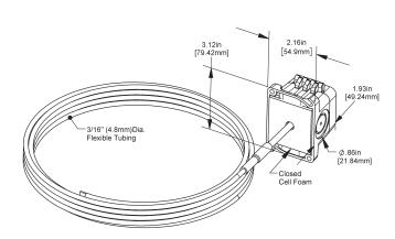
Fig. 1: Duct Averaging Unit with BAPI-Box Crossover Enclosure
