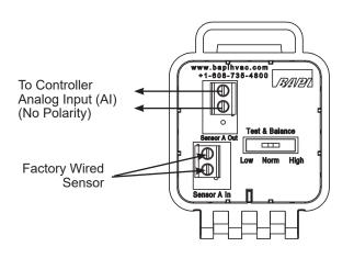
Fig. 10: Terminal Strip (-TS) or Test and Balance (-TB) Option for 2 Wire Sensors
