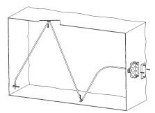
Fig. 9: Flexible Sensor Vertical Mount (Best for Horizontal Stratification)
