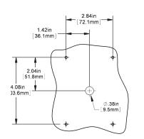
**Fig. 13:** BAPI-Box **(BB)** Enclosure Mounting and installation Holes (Rotate 90° for Horizontal Mounting)
