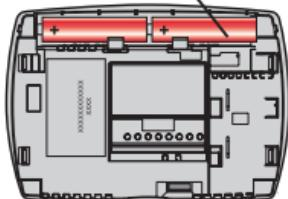
Batteries are optional (for backup power) if your thermostat was wired to run on AC power when installed.
