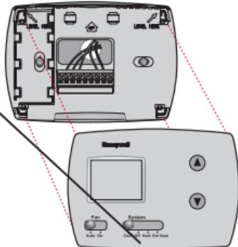
Turn thermostat over, insert fresh AA alkaline batteries, then reinstall thermostat.
