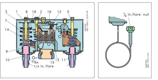
The switch in the KP has a snap-action function where the bellows move only when the cut-in or cut-out value is reached.
