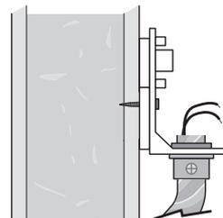
Sensor with wiring from bottom
