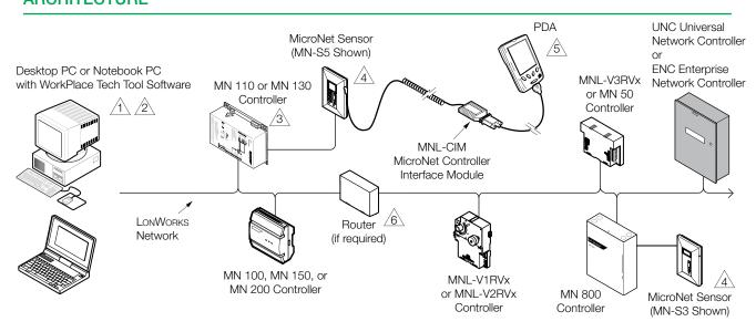
A PC can be connected to the LonWorks TP/FT-10 Network, either directly or through the LonWorks® network jack of a LonWorks controller or MN-Sxxx Wall Sensor. The PC must have an Echelon® LonTalk® adapter.
