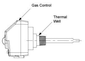
Step 5. Remove gas control & thermal well by rotating flats of Thermal Well counter clockwise (1-5/16"wrench).
