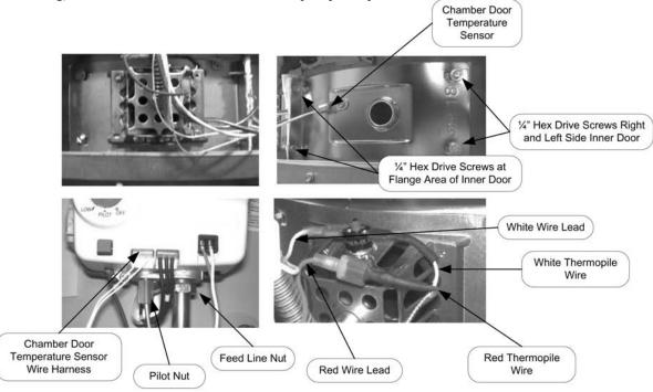
Step 4. Fully inspect burner and inner door gaskets for the following:
