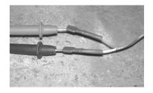
Step 3. Following the lighting instruction label on the heater, proceed to light the pilot and allow to operate for three minutes. It will be necessary to hold gas control knob down in the "PILOT" position continuously throughout this test. Any reading over 400 millivolts indicates good thermopile output.
