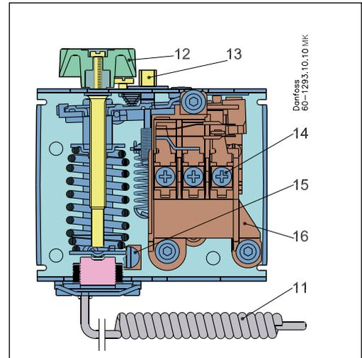
Switches in KPU controls have a snap-action function, triggered when cut-in or cut-out temperature is reached.
